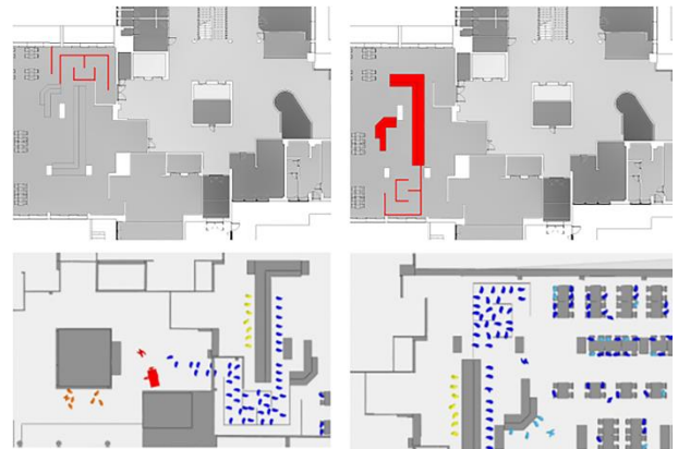
Figure 7 Crowd simulation of the current in-use scenario applied to low-budget reconfigurations
