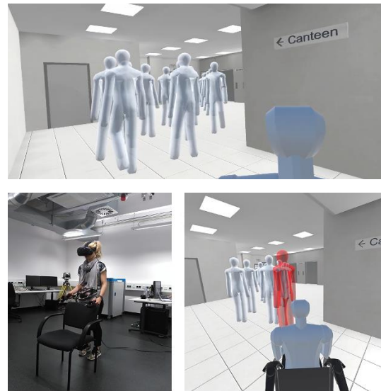
Figure 12 Circulation path from the emergency entrance and the elevators is simulated from the perspective of a person pushing a wheelchair
