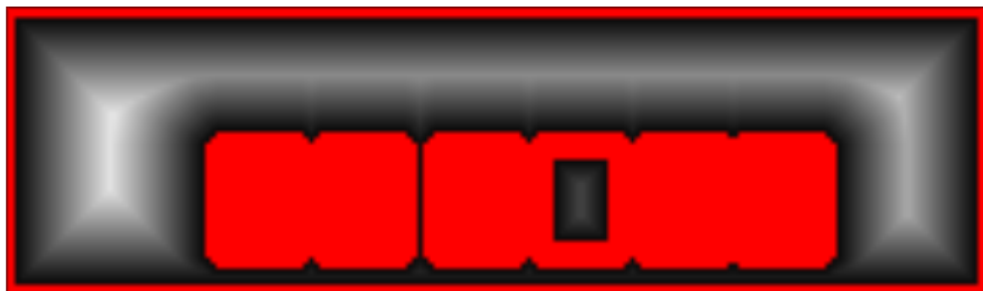
The resulting obstacle map shows the first and last barriers are below and above the cutoff. The 5th barrier has top and bottom beyond the cutoff so only the walls are included.
