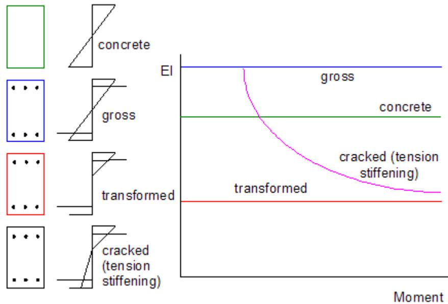
For a symmetric section, symmetrically loaded, stiffness can be expressed as
