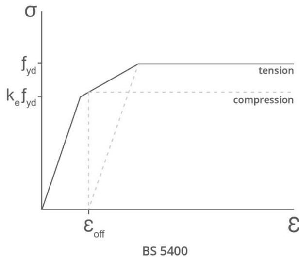
In tension the initial slope is defined by the elastic modulus,  $E$ , until the stress reaches  $k_e f_{yd}$ . The slope then reduces until the material is fully plastic,  $f_{yd}$ , at  $\epsilon = \epsilon_{off} + f_{yd}/E$ . Post-yield the stress remains constant until the failure strain,  $\epsilon_u$ , is reached. For BS5400  $k_e = 0.8$  and  $\epsilon_{off} = 0.002$ .
