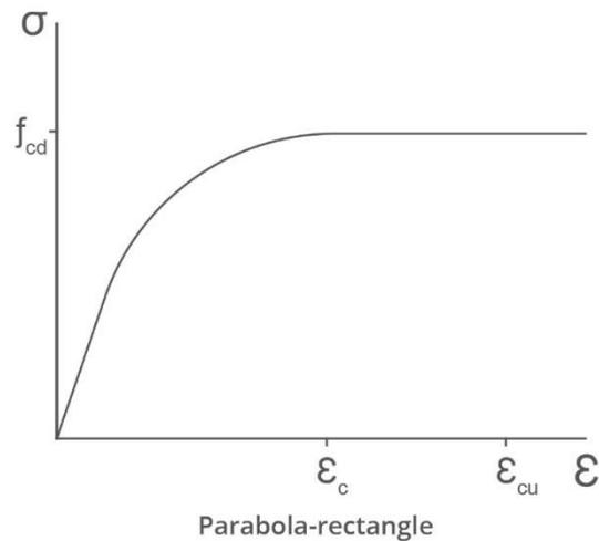
The parabolic curve can be characterised as
