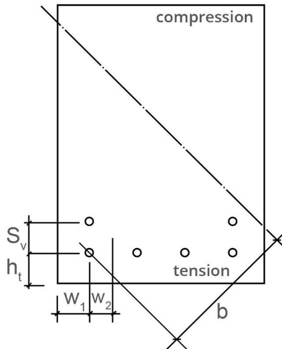
The first stage is to identify the most tensile bar and determine the cover  $c$  to this bar. We then define  $h_t$  as the cover plus half the bar diameter.
