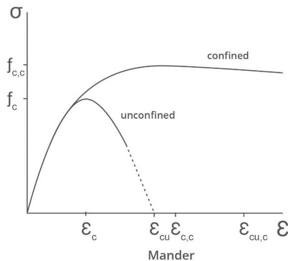
For unconfined concrete, the peak of the stress-strain curve occurs at a stress equal to the unconfined cylinder strength  $f_c$  and strain  $\epsilon_c$  generally taken to be 0.002. Curve constants are calculated from
