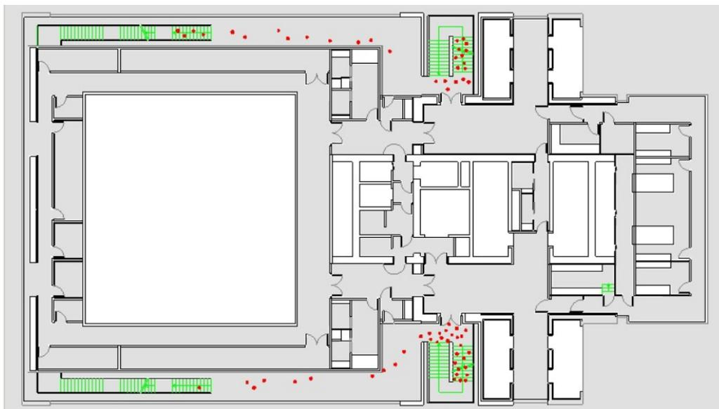
**Figure 5: Occupants flow through the “transfer corridors”**
