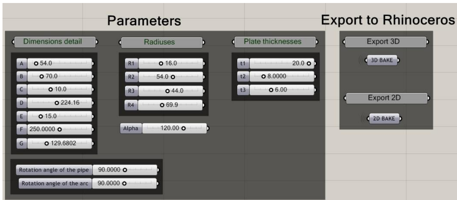
Figure 11. Generative modeling template of detail column connection.
