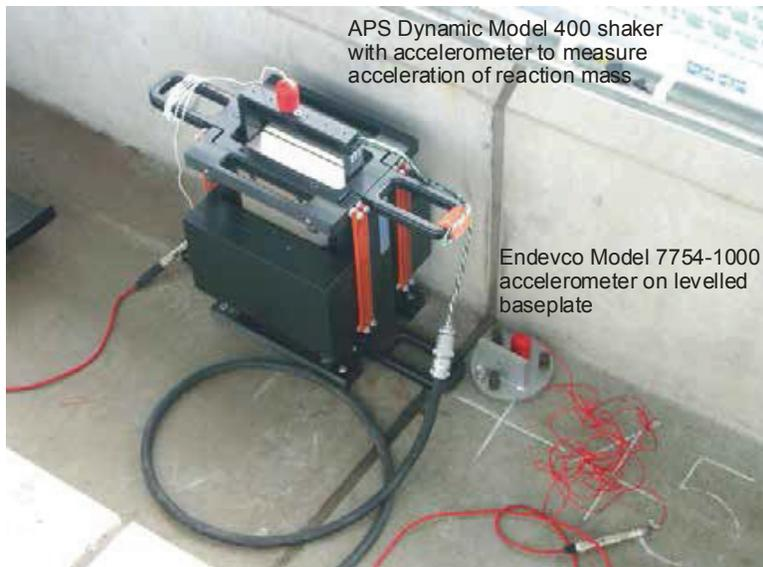
**Figure 7: View of Shaker and Accelerometer.**
