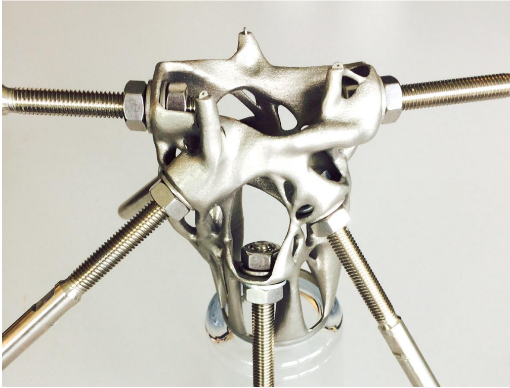
Figure 10: Image from the stainless steel AM node with connecting threaded swaged ends to the cables, the light armature and strut are not present.
