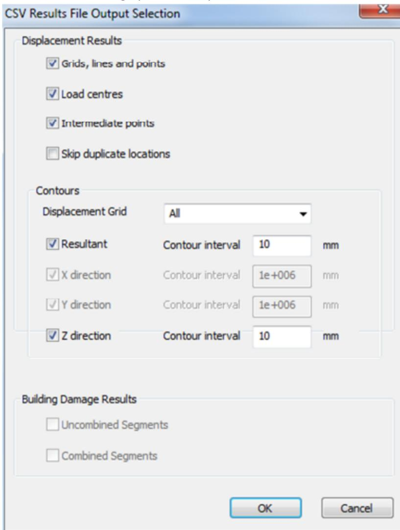
(Note: X and Y settlements are not shown as these are not calculated for the Boussinesq method)
