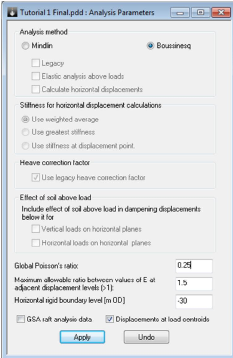
(Note: The horizontal rigid boundary level sets the base of the analysis as where there is no settlement. This is often specified as the level of bedrock)
