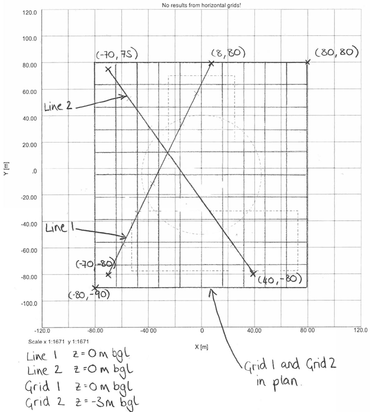
7. Double click on *Graphical Input* in the Gateway to check the load, displacement grid and displacement line geometry.
