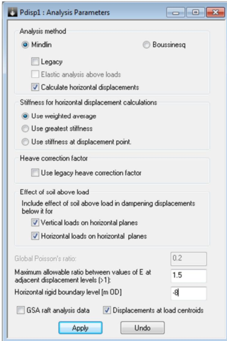
(Note: The legacy correction factor has not been chosen as the program defaults to the new correction factor, which is outlined in Section 2.3.2 of the User Manual)
