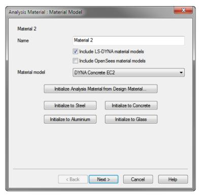
This leads to a page where the data to define the model can be entered. All parameters are defined as in the LS-DYNA Keyword Manual.
