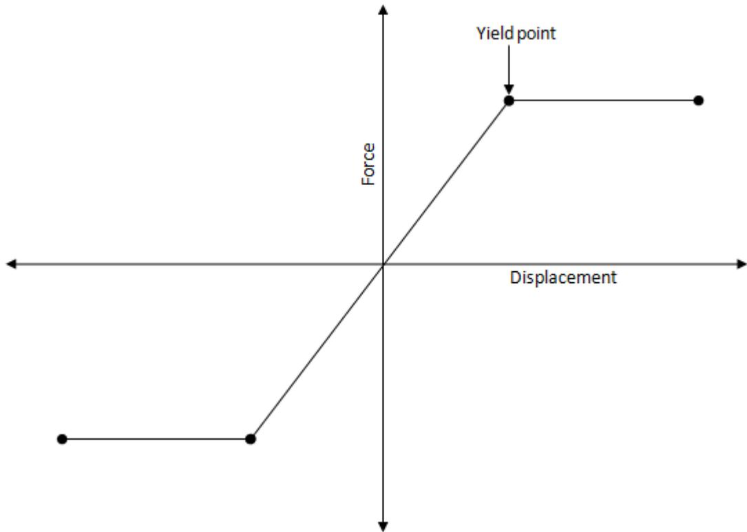
Typical elastic-plastic tip load load curve is shown below:
