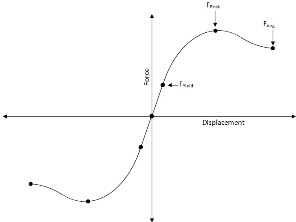
For the linear elastic zone the stiffness of the soil spring is given by:
