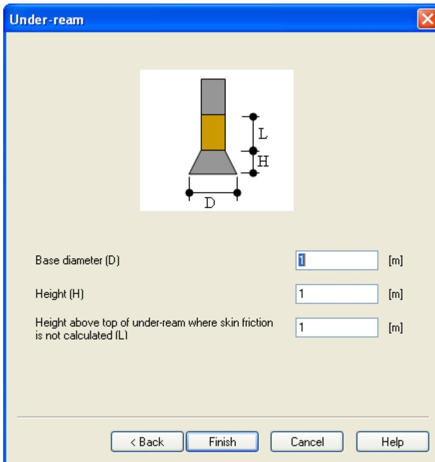
The **Under-ream** dialog box contains a diagram of a tapered shaft and three input fields. The diagram shows a shaft with a base diameter  $D$ , a height  $H$  for the under-ream section, and a height  $L$  above the under-ream section. The input fields are:
