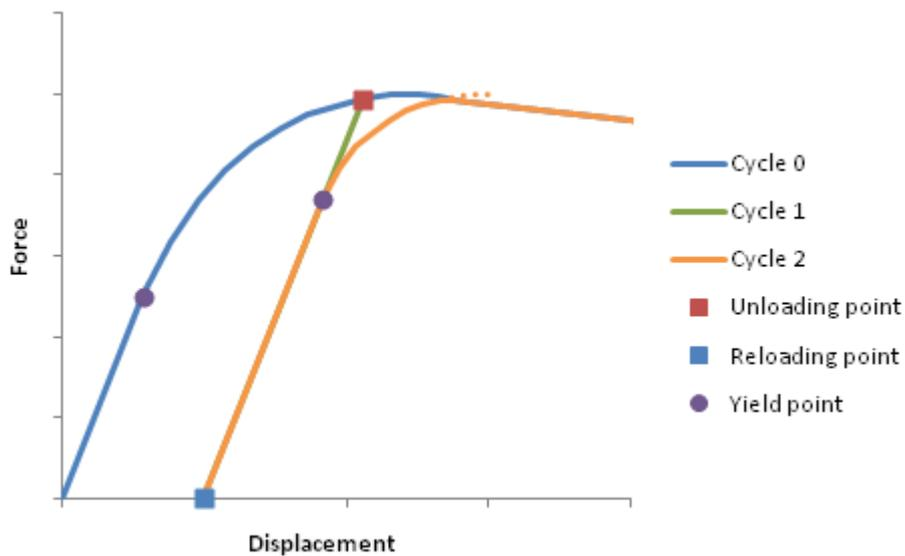
As can be seen from the graph above, cycle 2 is limited by the initial monotonic curve i.e. blue
