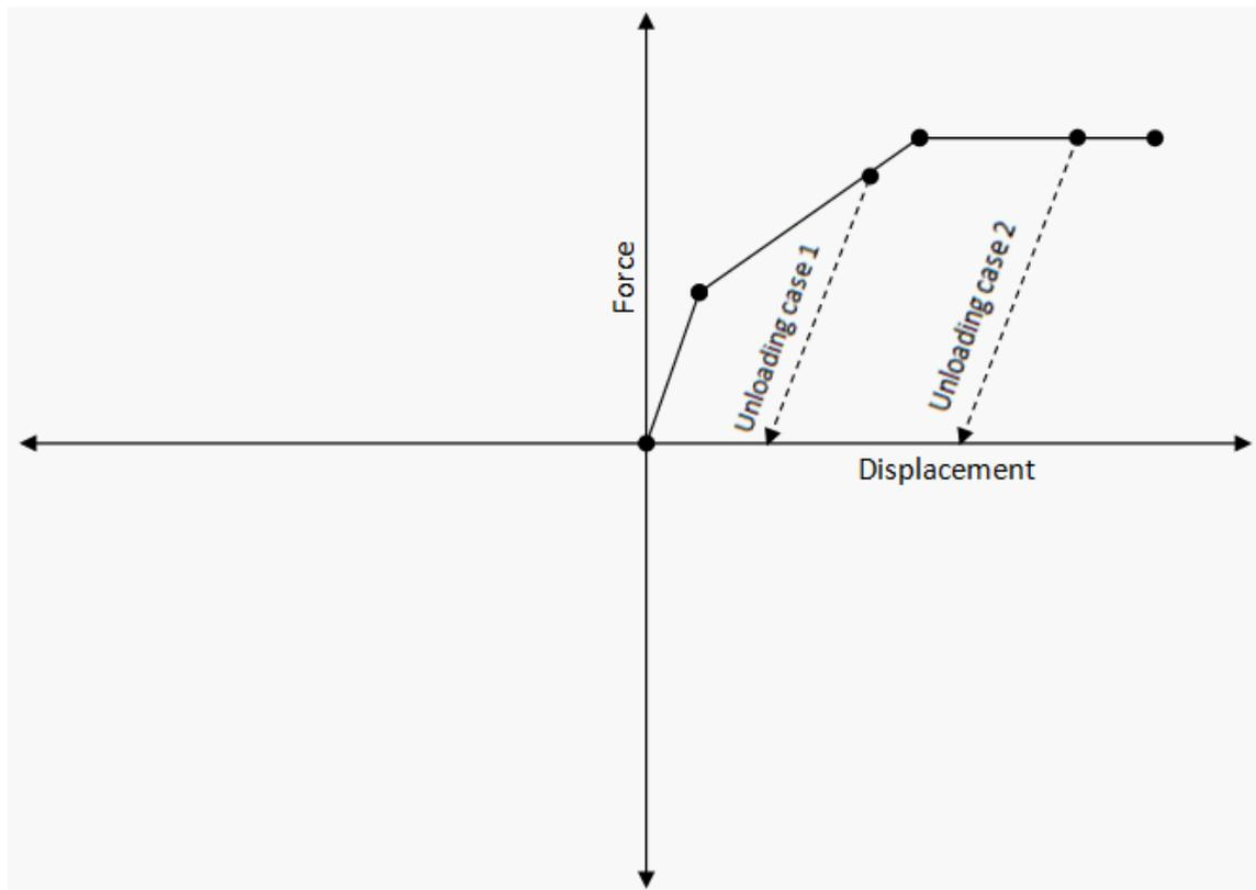
As a result, all the points on the unloading side of the curve shift parallel as shown below:
