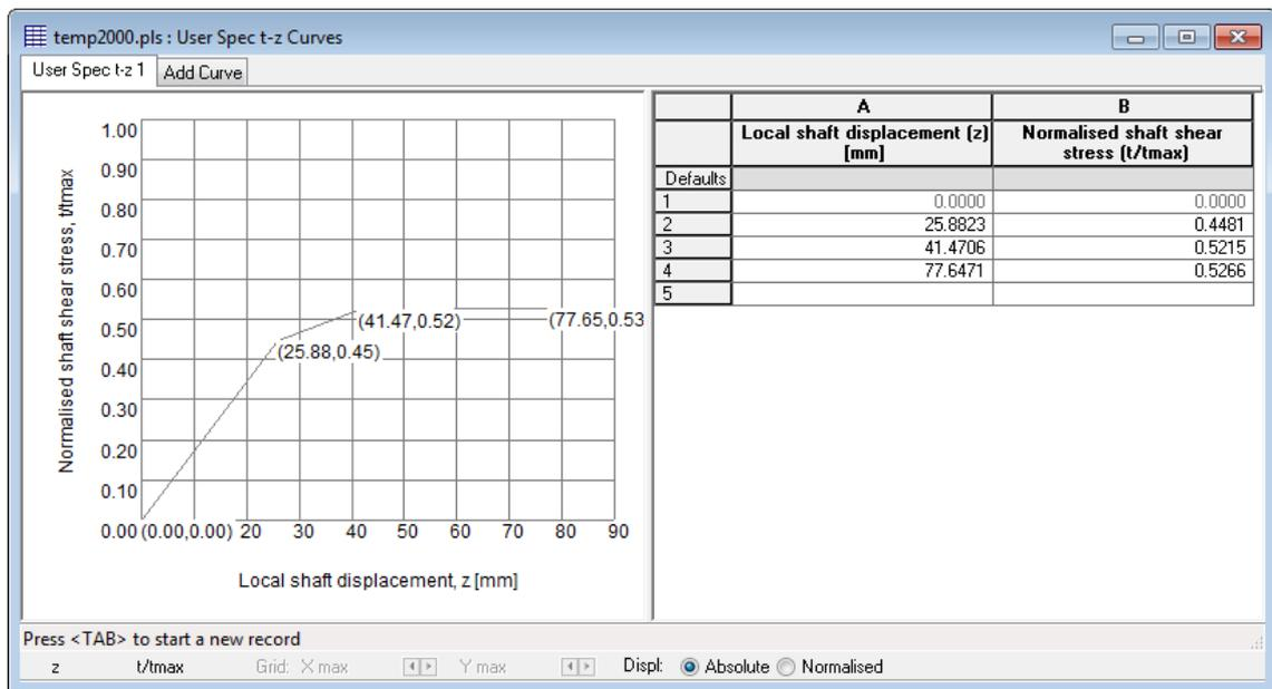
**Local shaft displacement z** - the shaft displacement. This can also be normalised by selecting the normalised radio button. By default, it is absolute.
