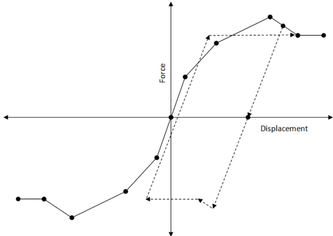
As can be seen from the figure above, when the spring is loaded into the post-peak softening zone, the peak strength for the subsequent stage is reduced to the value of the current force in the spring. In the subsequent stage also, if the spring is loaded into post-peak zone, there is a further reduction in strength i.e. peak force. This reduction continues until peak spring force falls to residual value. Thereafter, the behaviour is similar to the non softening case described above.
