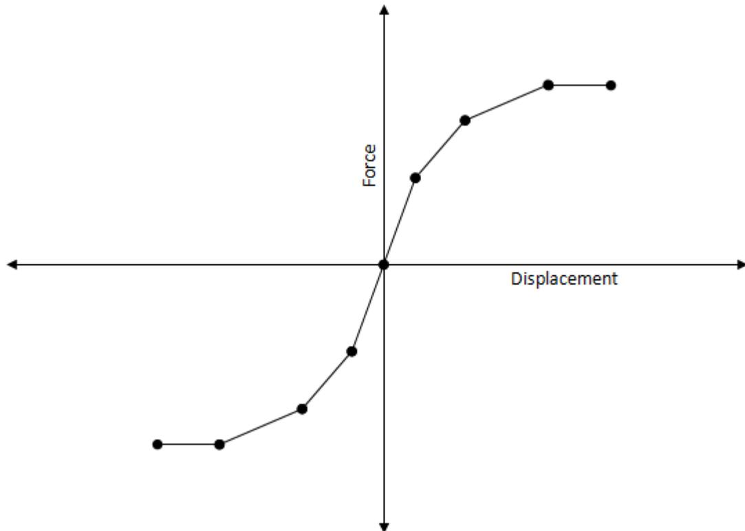
For the base curves too, the user is required to enter a series of points as discussed above. However, the curve is not extended into the tension region i.e. base spring does not take tension.
