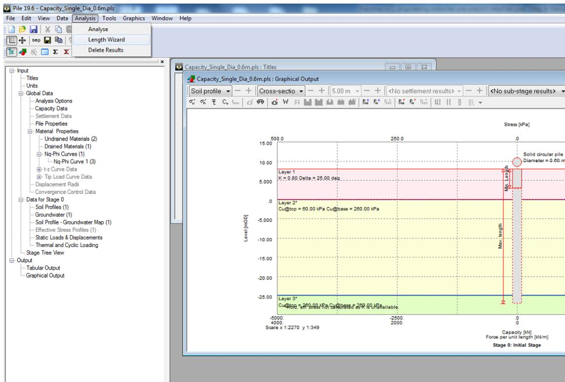
After this dialog is invoked, the user needs to enter the soil profile, and pile cross section of interest, and then press the "Calculate" button to view the result.
