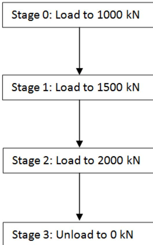
During analysis, when the program encounters a stage that has cyclic loading specified for 'N' cycles, it generates  $2N+1$  sub-stages as shown below:
