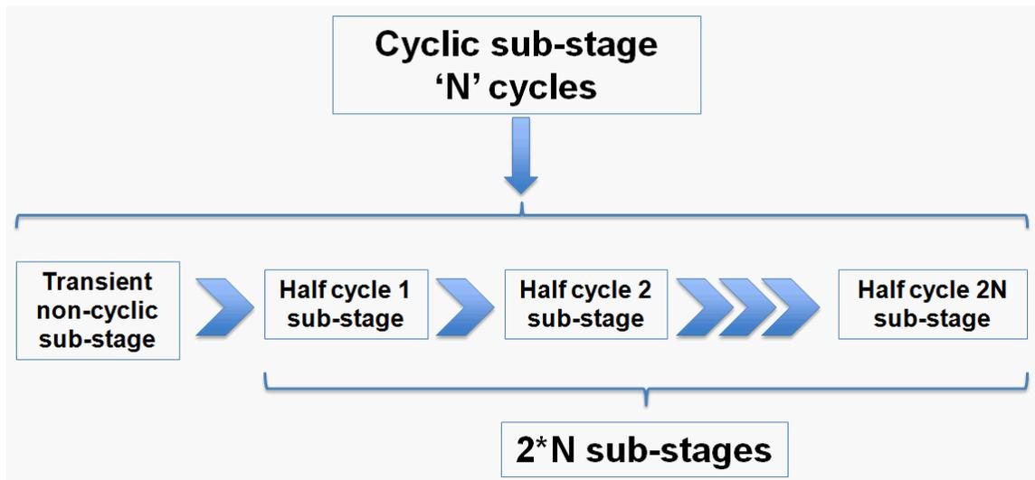
The transient sub-stage is inserted to explicitly apply non-cyclic loading component of the original loading stage. Then, in the subsequent sub-stages, additional cyclic loads are applied.
