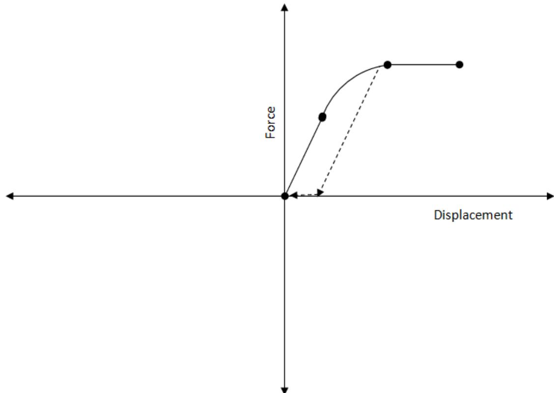
The pile base shows a response that is parallel to the initial elastic gradient on unloading, with no tension capability. Upon reloading, the displacement accumulates with no load carried until it reaches the elastic unloading path, retraces the unloading path in the opposite direction up to the updated yield stress on the initial loading path (as tracked using assumptions described for shaft curves), then follows the updated loading path to peak stress.
