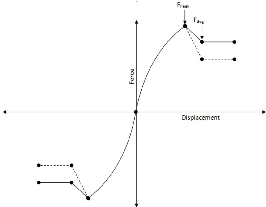
For base interaction, there is only one type of curve - same for both clay and sand. This is modeled by 5 points as specified in the API documentation.
