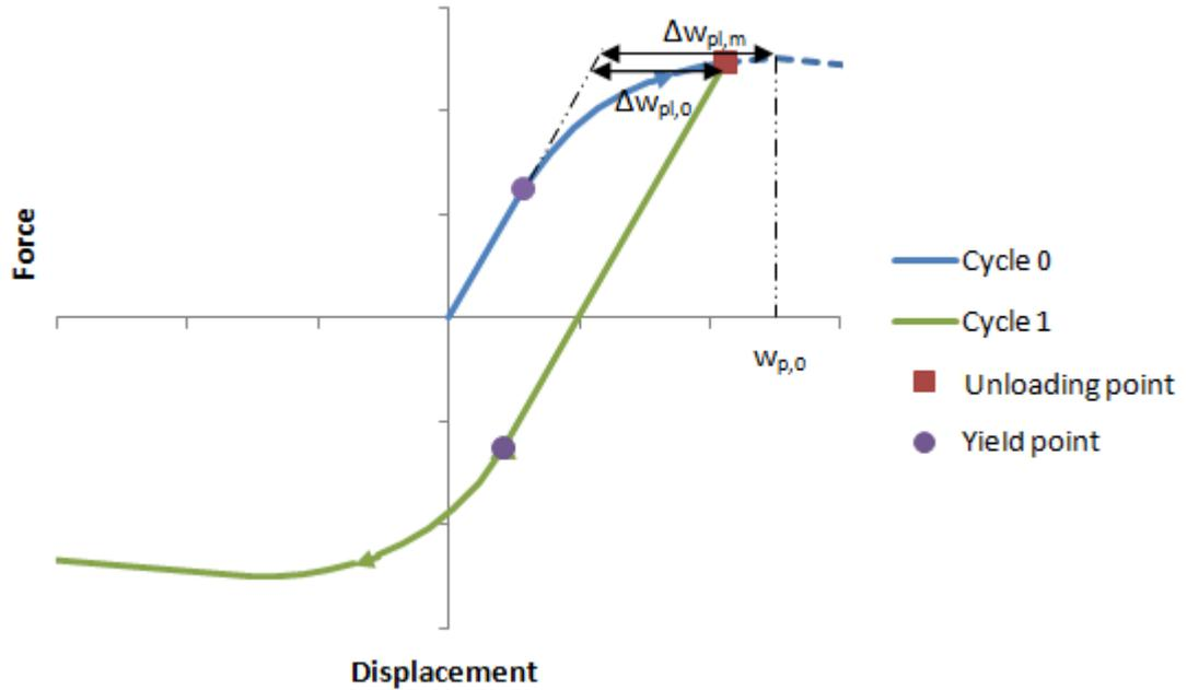
Also, the yield force in a particular stage (half cycle), depends on the spring force ( $f_{max}$ ) in the previous two half cycles (i.e. one tension stage and a compression stage).
