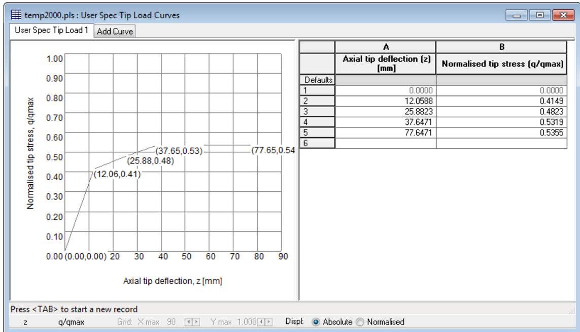
**Axial tip deflection z** - the deflection at the tip. It can also be normalised by selecting the normalised radio button. By default, it is absolute.
