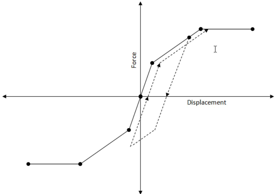
An alternative case where the the last load displacement curve shifts to the left of initial loading curve is given below:
