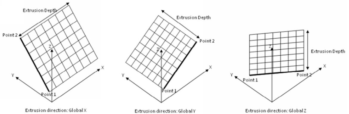
The extrusion depth should not be zero. Negative extrusion depth extrudes in the opposite direction to the global directions.
