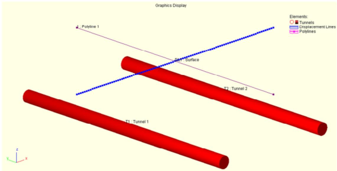
(Note: the polyline is only used for the generic building and utility damage assessments. The displacement line specifies the position of a specific building or utility.).
