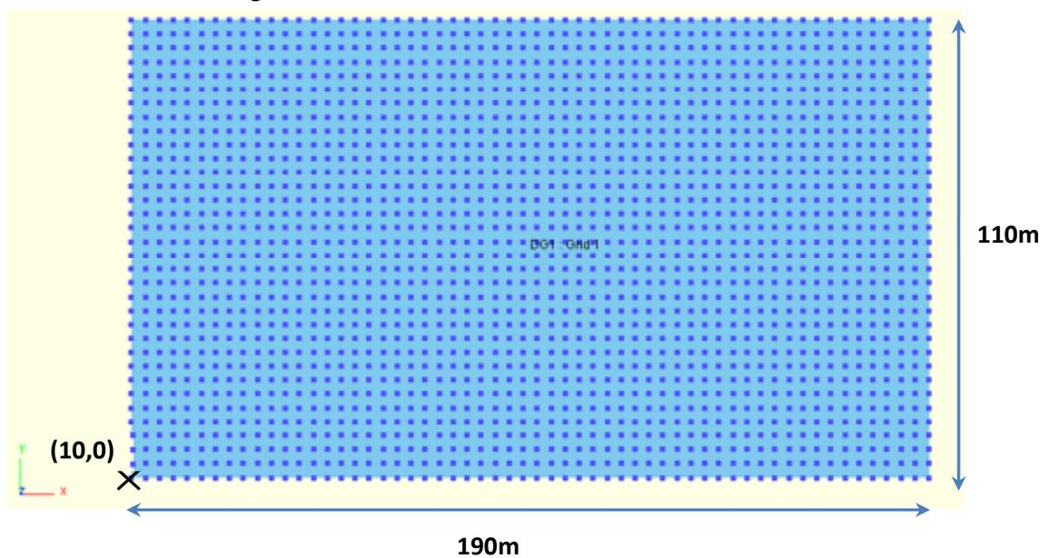
The grid should have 57 intervals in the x direction and 33 intervals in the y direction.
