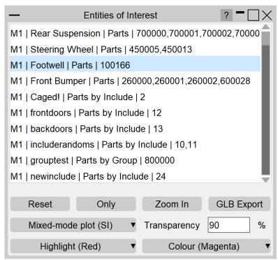
The image shown is an SI Mixed-Mode Plot on the Footwell and Coloured by Magenta on the Steering Wheel
