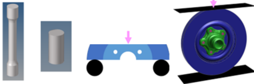
Tensile, Compression Coupon Tests, Brake Disc 3-Point Bend and Fully Bolted Crush Tests
