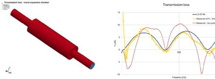
Fig. 4: Meshed model of round expansion chamber
