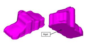
Figure 9 Boundary element model of oil pan
