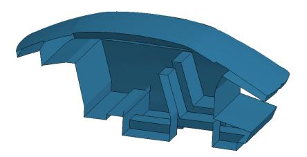
With FEM Acoustic solver in LS-DYNA, user can compute the noise distribution in a car cabin model, for each excitation frequency. The results are given by D3ACS, accessible to LS-PREPOST.
