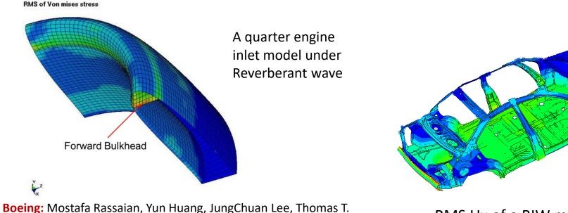
RMS Ux of a BIW model (by d3rms)
