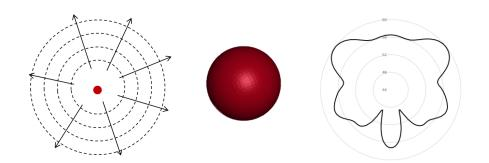
Acoustic scattering of a monopole incident wave on a rigid sphere
