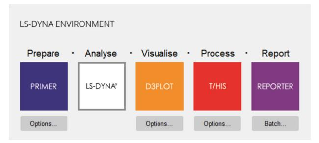
Select this option to access the PRIMER program. This program is a graphical model editor that will position occupant models, fold airbags and allow model parameters to be modified.
