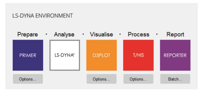
Select this option to access D3PLOT. This program is a graphical post-processor designed to access the binary output files created by LS-DYNA. For more details see the D3PLOT Manual.
