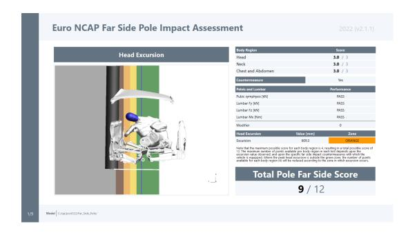
The template takes as an input the maximum intrusion data output from the updated <u>Side MDB and Side Pole</u> templates. It then calculates the maximum head excursion and produces a plot of the results, as well as calculating the total test score for either MDB or Pole.
