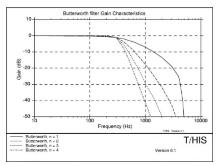
The cut-off frequency is the frequency at which the gain of the filter is -3dB (i.e. the magnitude of signals at this frequency is halved by the filter). The lower the frequency the less noise passes through; but any peaks in the signal tend to get reduced in magnitude and delayed in time.
