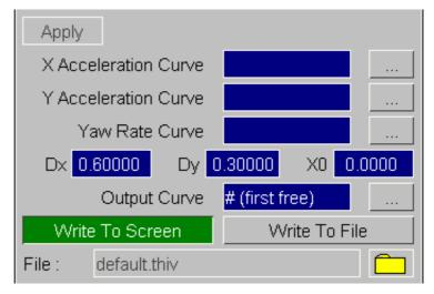
This option requires 3 input curves, a longitudinal and lateral acceleration and a rotation rate. The user is prompted for the constants Dx, Dy and Xo. See <a href="Appendix E">Appendix E</a> for more details on these calculations.
