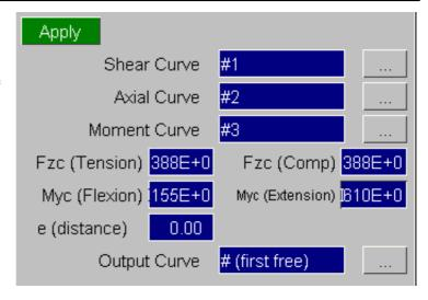
This option requires 3 input curves. 1 to represent Shear force, 1 to represent Axial force and a third to represent bending moment in the dummy's upper neck loadcell. Enter these curves in the corresponding input boxes.
