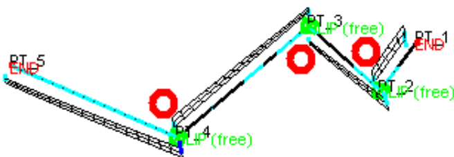
Belt passing over rollers, using "free" slippings at roller locations.
