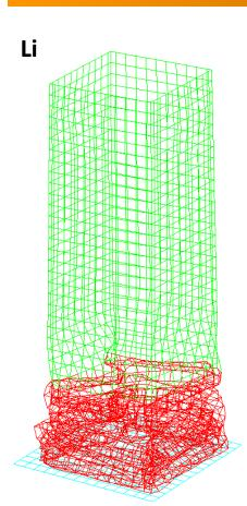
**Li** (Line) plot mode draws the current state in wireframe mode. Wire-frame mode exposes lines which should be hidden.
