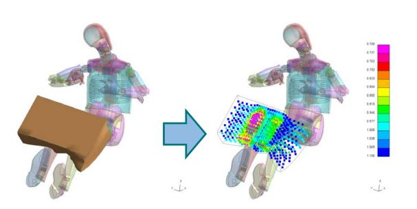
To change the way the points are displayed in the **CL** plot mode, under the Contour Options menu, select the Cloud Plots tab. Under this tab there are various options which allow the user to change the display for the **CL** plot mode.
