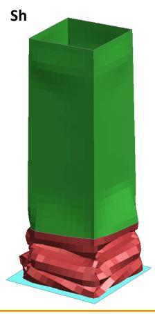
**Sh** (Shaded) plot mode draws the current state in lit and shaded "greyscale" mode, implicitly with hidden surfaces removed. Hidden lines are removed in this plot mode. When in the **Sh** plot mode, pressing the '**Y**' button on a keyboard will show the mesh of the model.
