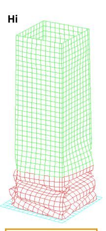
Hi (Hidden Line) plot mode draws the current state in hidden surface mode. Hidden lines are removed in this plot mode.
