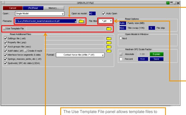
Filenames for the model file to be opened can be typed into the text entry box or the folder button can be used to search for the required model file. Recent files can be found in the drop down menu.
