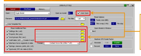
The Read Additional Files panel allows additional files to be read. With the Auto Open option selected, D3PLOT automatically selects these additional files to be read. Deselecting the Auto Open option, allows the file names of the additional files to be modified and allows the user to manually search for a particular additional file.
