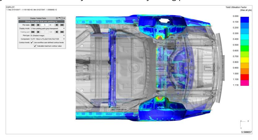
\*Note: Yielding parts are parts containing at least one yielding element, measured as an element with a <u>Yield Utilisation Factor</u> greater than one (or <u>Yield Utilisation Percentage</u> greater than 100%).
