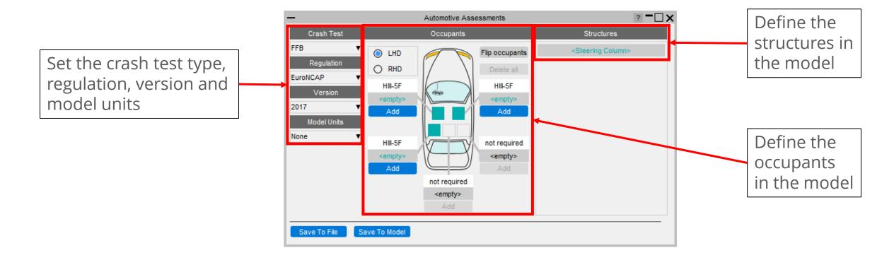
The Occupants section is used to select which occupants are in the vehicle, their positions in the vehicle, and the IDs of the entities from which data can be read.
