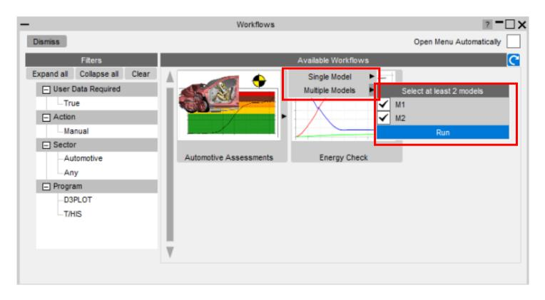
• When launched in D3PLOT, the Automotive Assessments Workflow will extract the data required for the assessment and process it according to the rules set out in the
