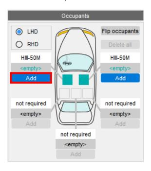
2. This will open a window where you can select the occupant type. Input entity IDs are filled automatically from a list of popular suppliers.
