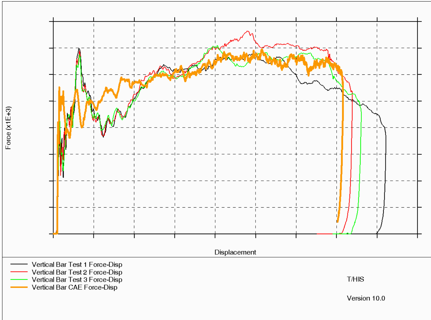
Figure 1.16 – ODB Test E Force – Deflection Curve (C60)
