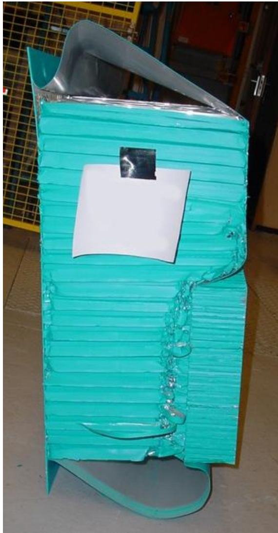
Figure 1.3 – ODB Test A final deformation
