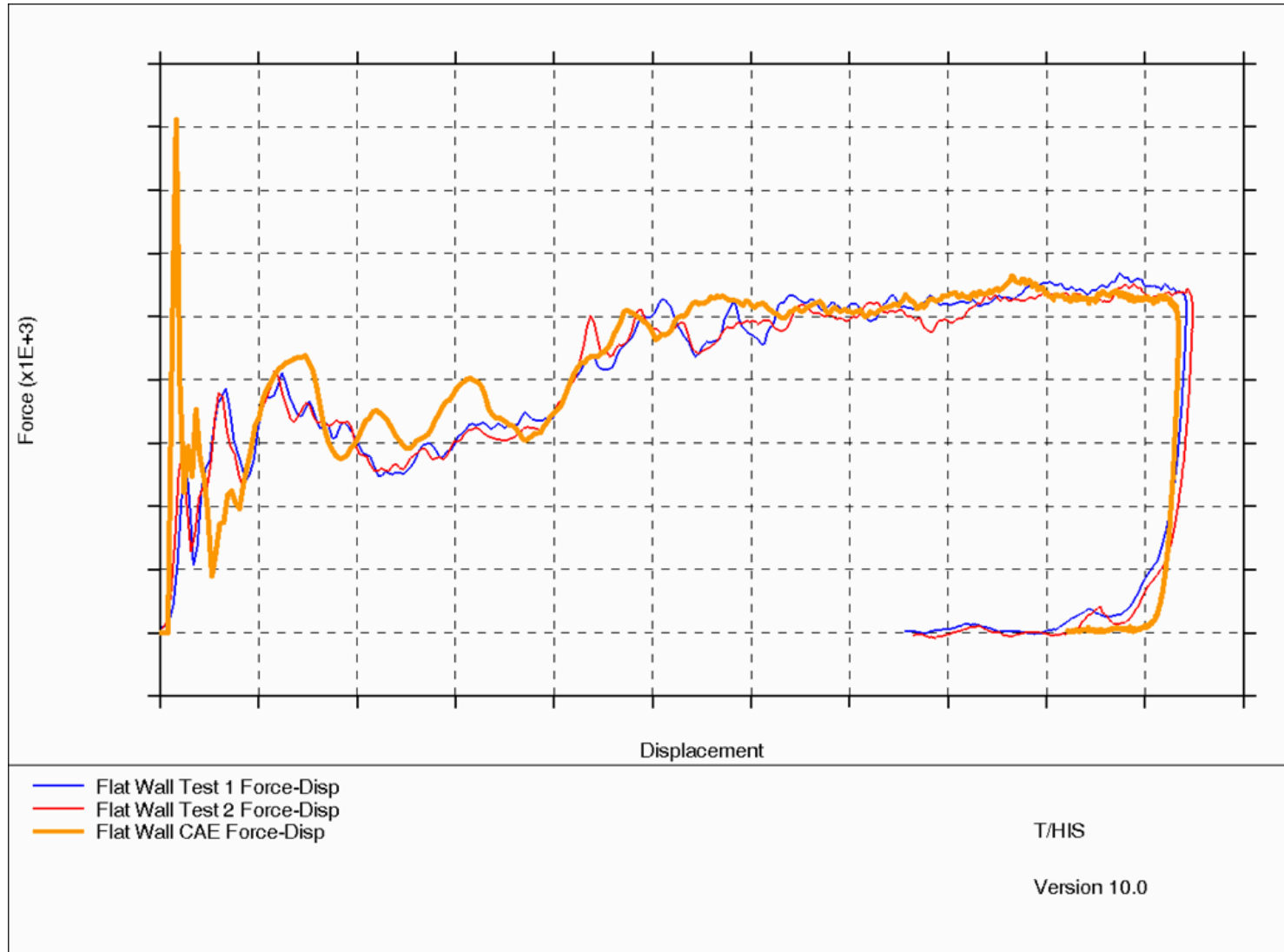
Figure 1.4 – ODB Test A Force – Deflection Curve (C60)
