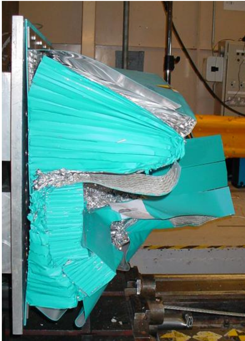
Figure 1.9 – ODB Test C final deformation
