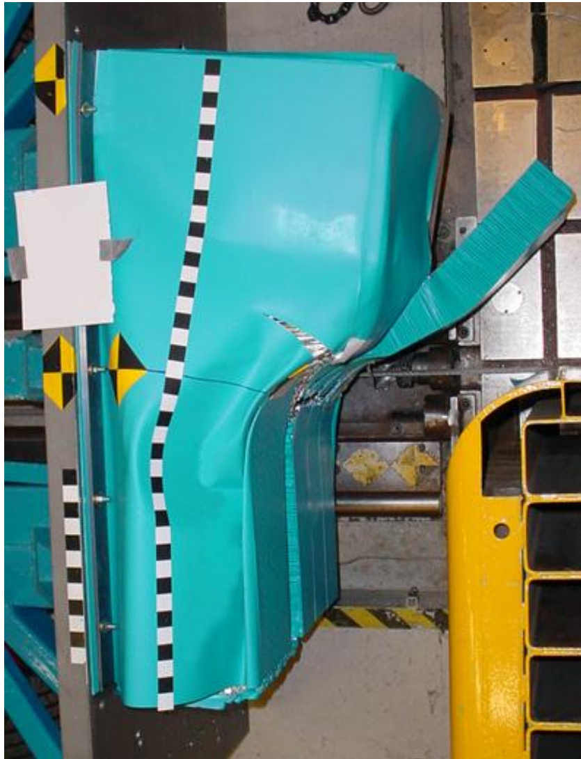
Figure 1.6 – ODB Test B final deformation
