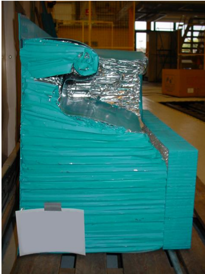
Figure 1.12 – ODB Test D final deformation
