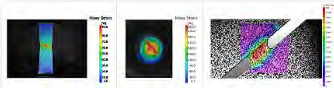
Tensile, biaxial, and grooved shear tests for GISSMO failure modeling
