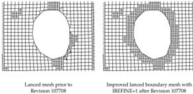
Figure 2. Set IREFINE=1 for mesh refinement along the lancing curve.
