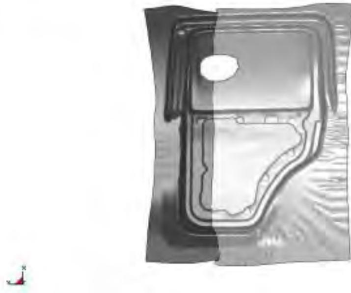
Figure 1. Lancing across a laser welded line.
